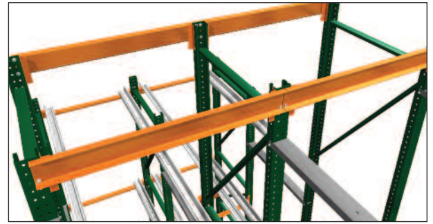
Bolted-In Top Braces - Tie the uprights together for increased system rigidity and stability.
